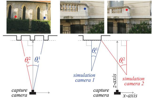
**Figure 2:** Left: Top-view of capture camera and two eccentricity angles,  $\theta_e^1$  and  $\theta_e^2$ . Right: two simulation cameras, their simulation angles  $\theta_s^1$  and  $\theta_s^2$ , and corresponding virtual images. See how simulation angle affects final image quality. Depending on which corner we look at, eccentricity also affects distortion.
