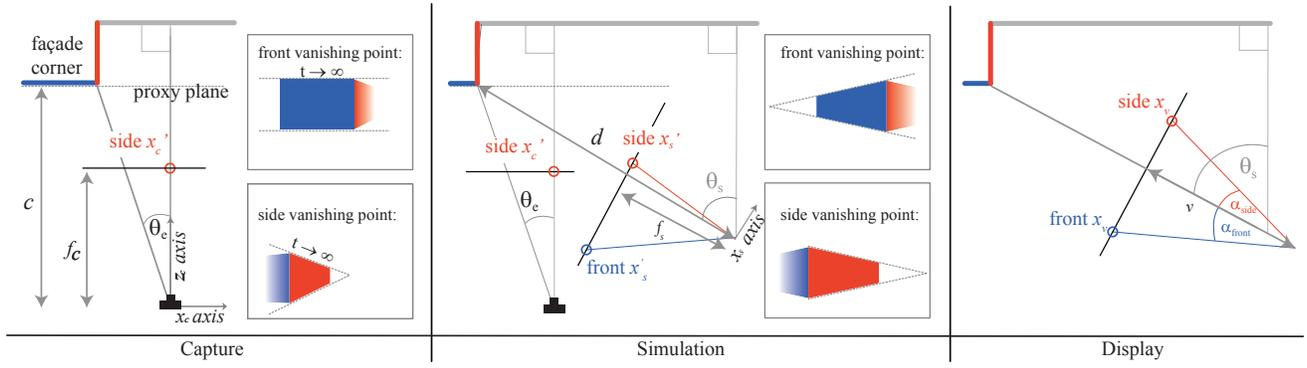
**Figure 3:** Left: Top view of capture camera geometry; the insets show the vanishing points (VPs) as seen in the screen for front and side of balcony. Middle: Top view of simulation camera geometry: again insets show vanishing points. Right: Top view of display geometry.
