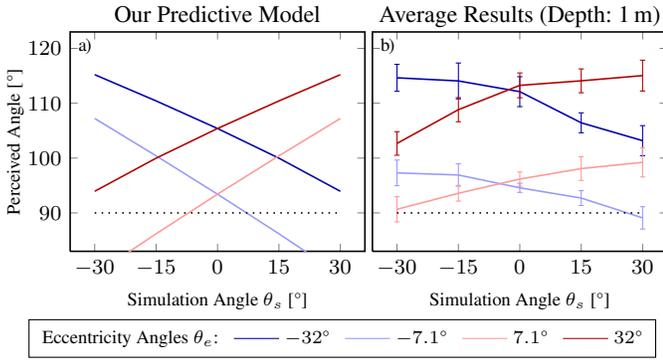
**Figure 10:** Our predictive model (a) compared to the hinge angle-matching results (b), both for façade depth of 1 m. Each line corresponds to an eccentricity angle; error bars indicate one standard error about the mean. The dotted line at 90° is the scene hypothesis.
